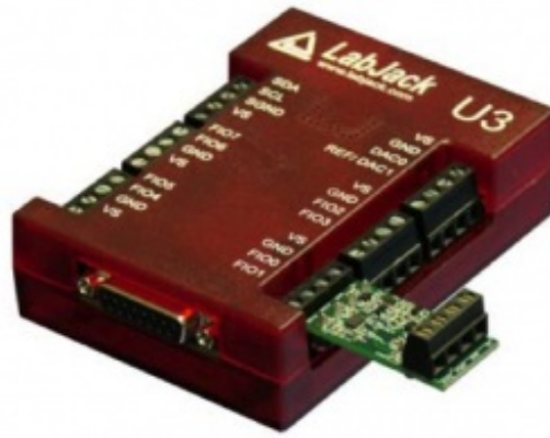
Figure 2: LJTICK-DAC With U3
