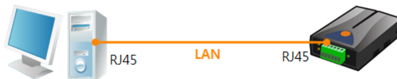
Figure 2-1 the connection between CIE-H12 and a PC
